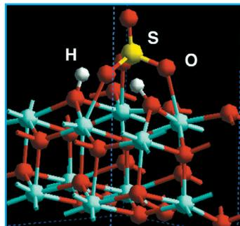
▲ An example of  $H_2SO_4$  dissociative adsorption analysis on the tetragonal(101) face of  $ZrO_2$
